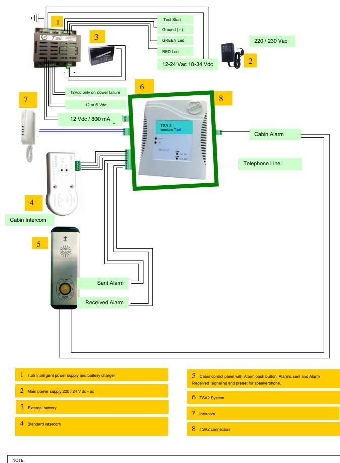
Alarm input can be set N/O or N/C. Sent and Received alarms are relay contacts.
