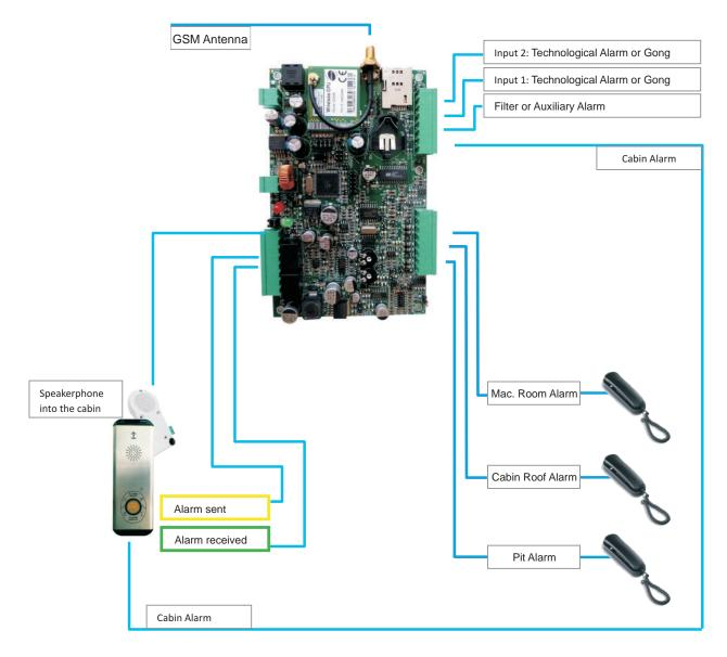
Where to install Power Supply Power consumption max. (@12 Vdc) Power consumption min. (@12 Vdc) Relay contacts flow GSM frequencies Dimensions Weight Machine Room, On Cabin Roof or everywhere there is good GSM signal 10 ÷ 16 Vdc 300 mA 30 mA 3A @ 120 Vac / 3A @ 24 Vdc 800/900/1800/1900 MHz 165 x 184 x 35 mm 200 g
