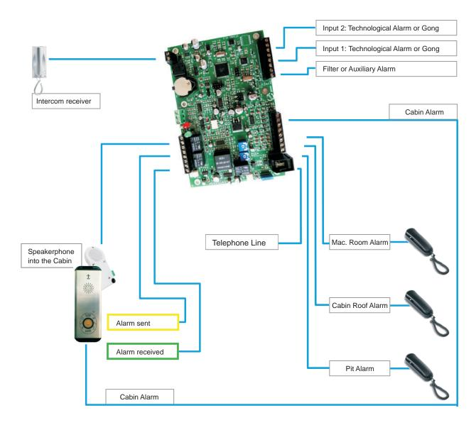
Where to install Power Supply Power consumption max. (@12 Vdc) Power consumption min. (@12 Vdc) Relay contacts flow Dimensions Weight Machine Room, Fixed to the wall, On Cabin Roof 10 ÷ 16 Vdc 240 mA 30 mA 3A @ 120 Vac / 3A @ 24 Vdc 165 x 184 x 35 mm 200 g
